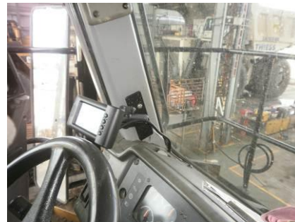
Figure 7: Operator display mounting
